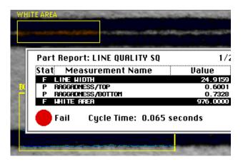
Figure 4a. Example of a line quality test report
