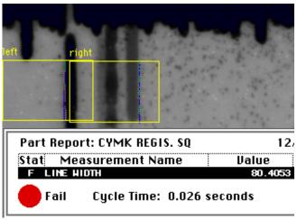
Figure 7. Color registration test
